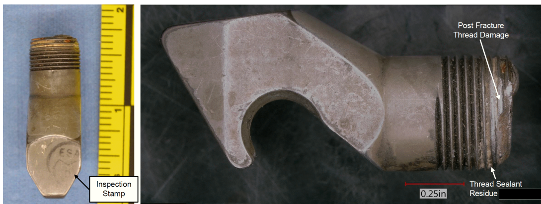
Figure 4: The fractured forward upper hook
