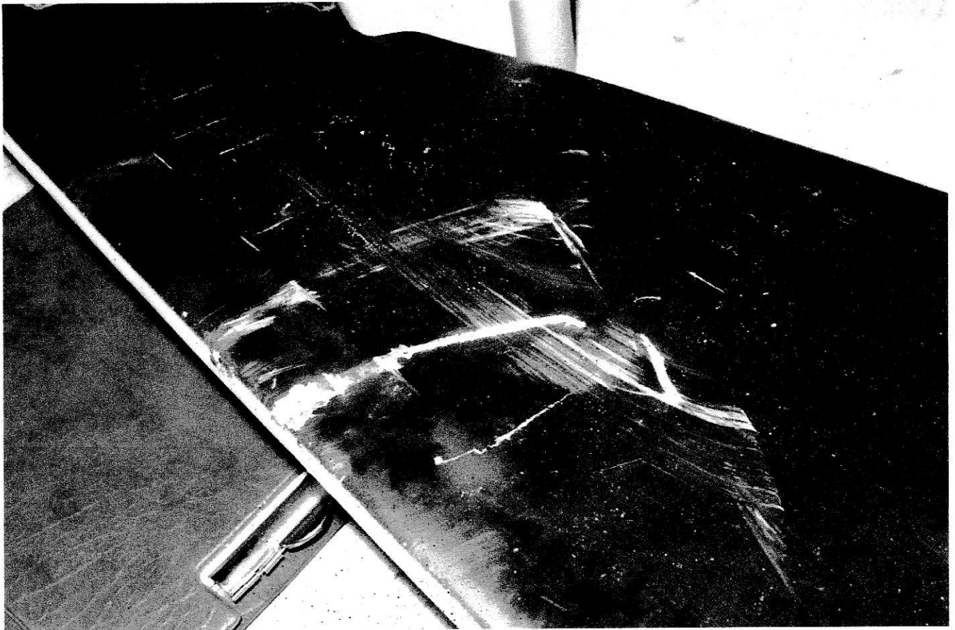
The black main rotor blade stub. View of the marks on the underside caused by the sliding door strike.
