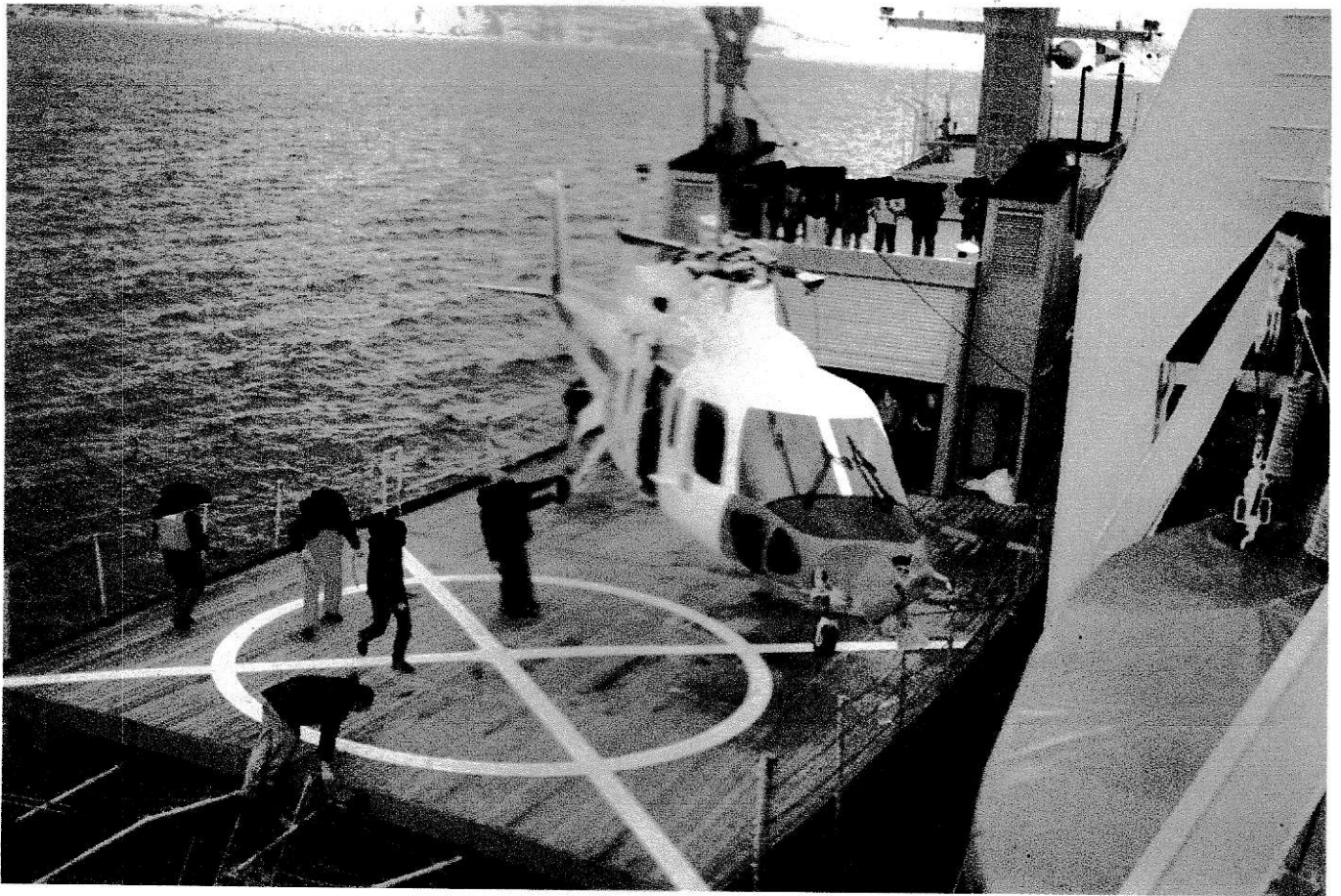
Wreck as recovered on the helideck of Okinawa . Chin and door windows broken and sliding door missing.
