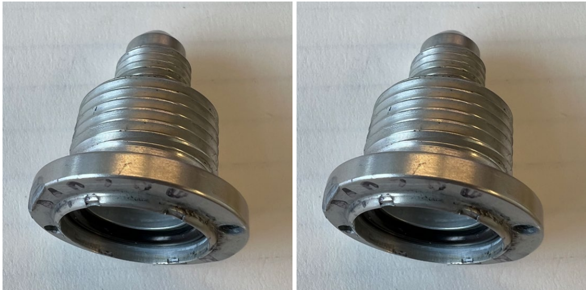
Figure 3: Right nacelle firewall fuel filter drain
