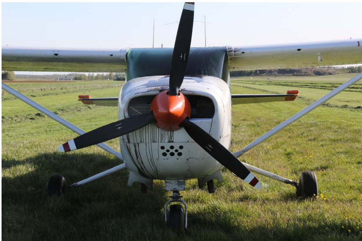
Figure 3: TF-MAJ oil leak blocked forward window vision
