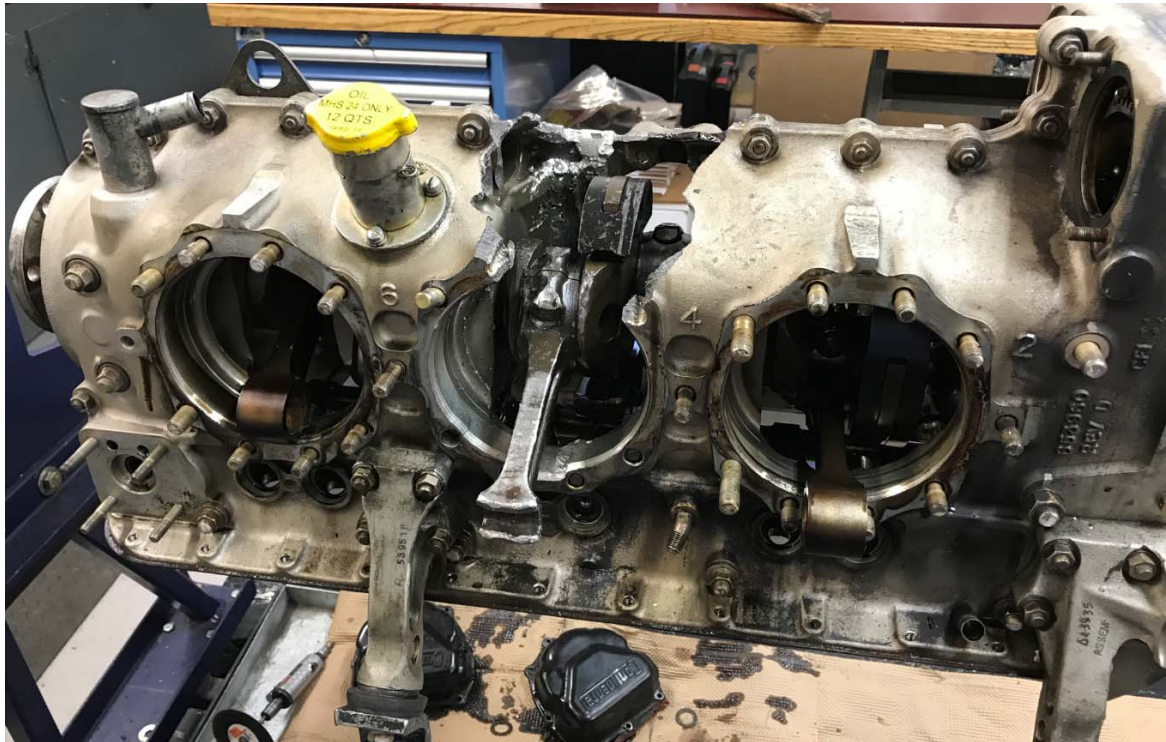
Figure 5: Engine S/N1012306 after the cylinders had been removed
