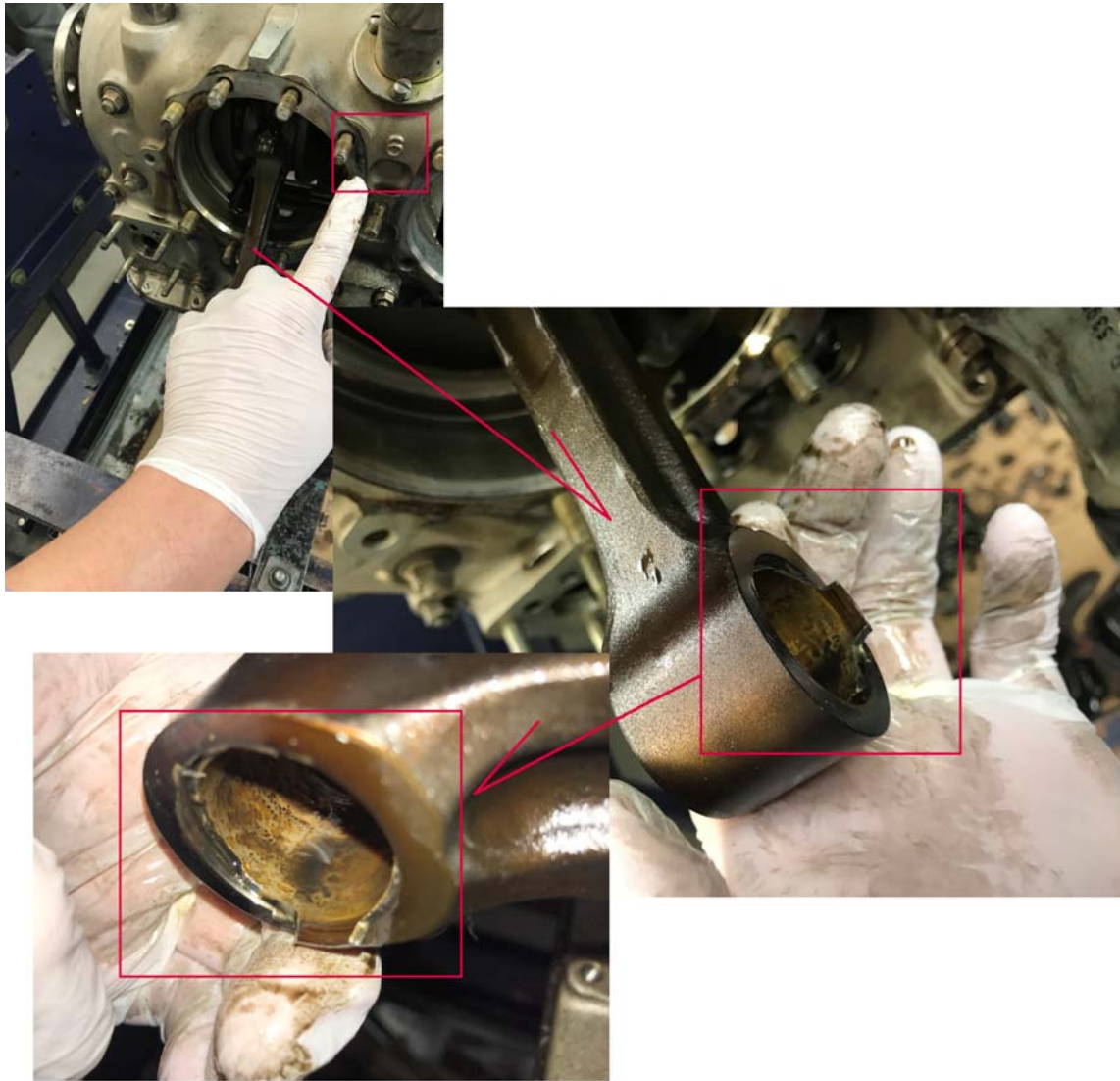
Figure 9: Connecting rod no. 6 (S/N AE15DA666) – Small end bushing migration and damage
