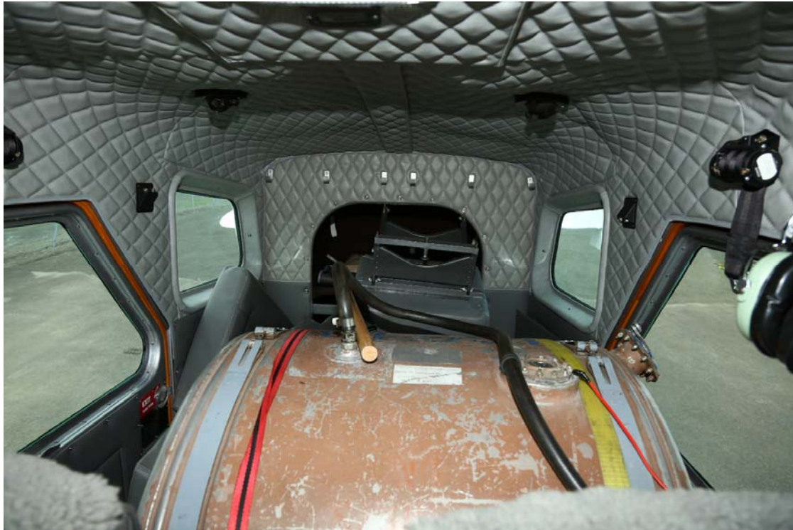
Figure 20: Picture showing the installed ferry fuel tank and the 2 nd seat row in the aft part of the cabin
