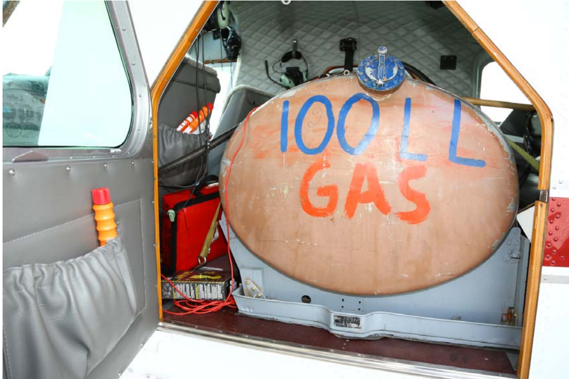
Figure 9: Ferry fuel tank installed in cabin, seen through left cabin door
