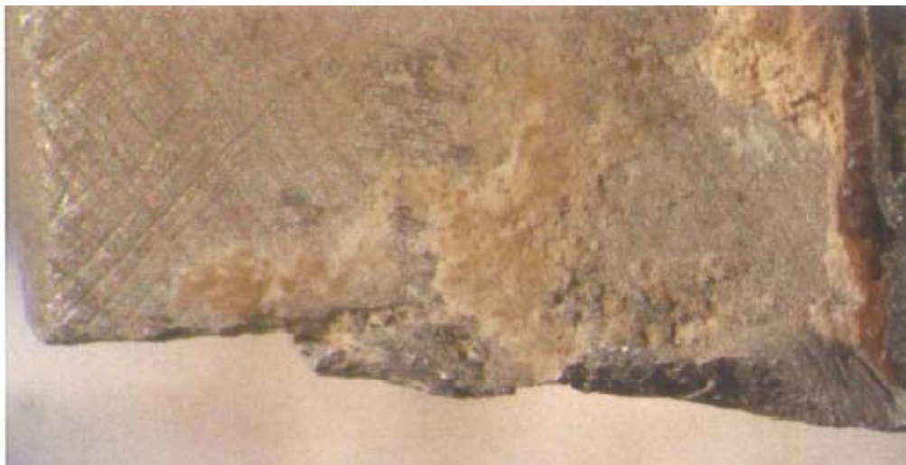
Figure 5: Position 1b seen from the side. Corrosion pits are visible on the surface.
