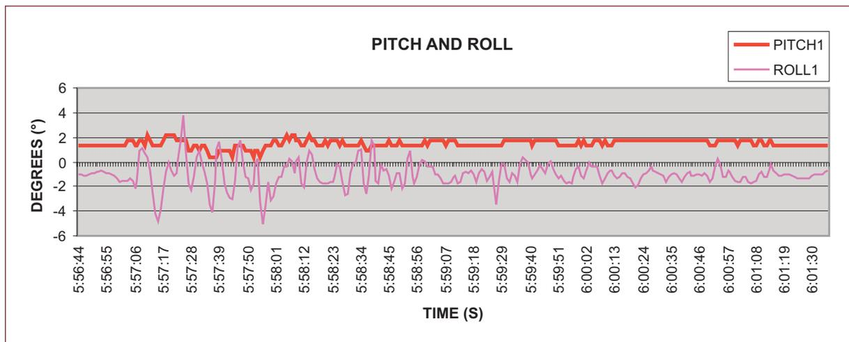
Figure 1.11.6. Pitch and lateral aircraft roll
