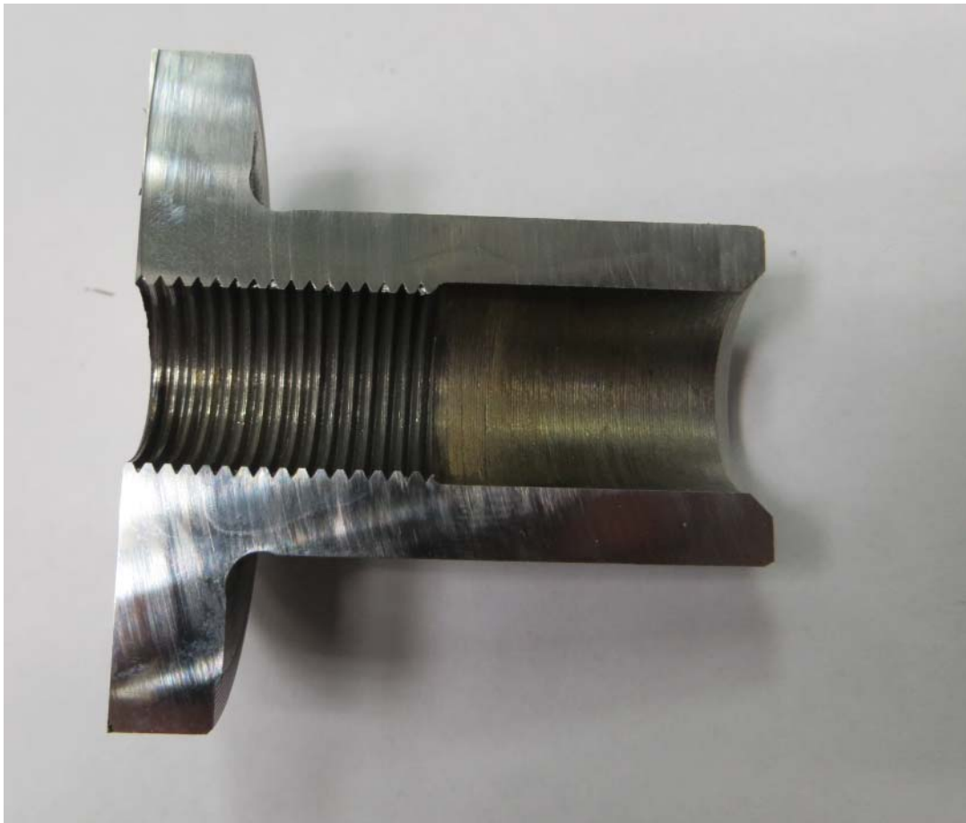
Figure 15: No damages found to fastener hole threads
