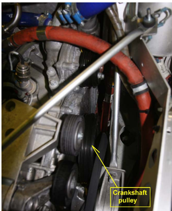
Figure 6: Crankshaft pulley skewed out of position
