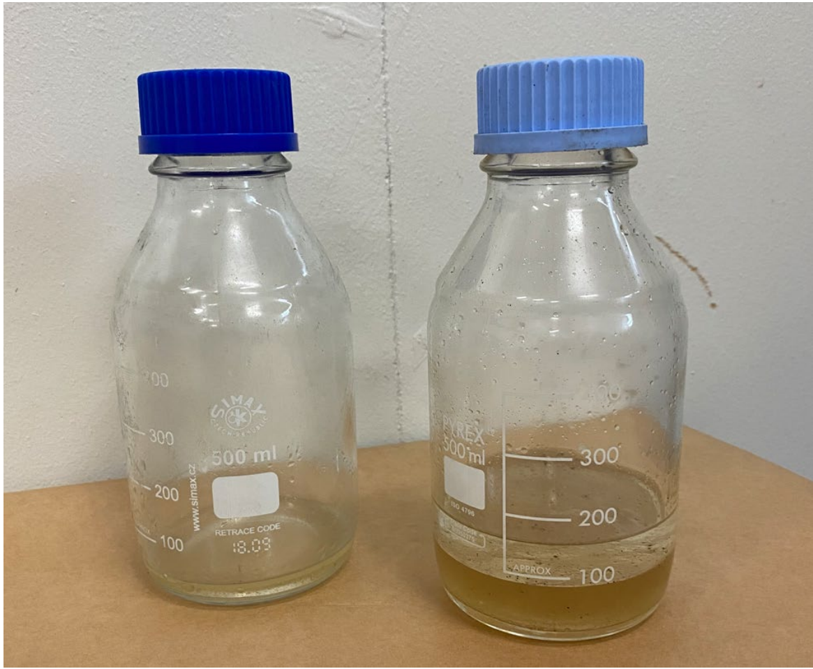
Figure 6: Fuel found contaminated with water
