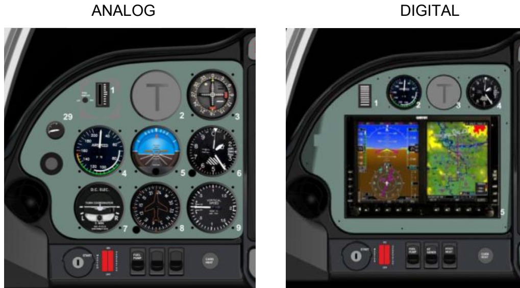
Figure 31: The difference between analog and digital panels
