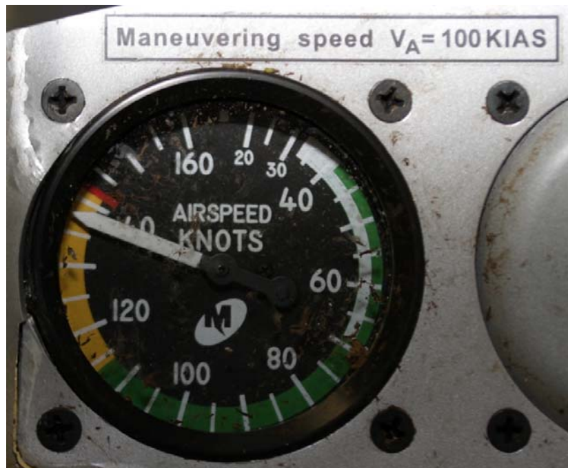
Figure 33: Airspeed indicator markings on instrument
