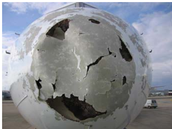
Figure 1 Damage to radome
