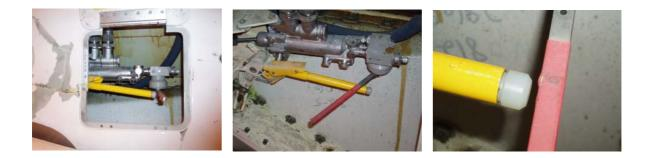
The red/actuator vent handle was turned 90 degrees outboard to the manual position to disarm the inflation system. It was necessary to raise the yellow/round crank handle to give the red/actuator vent handle space enough to be operated inwards.
