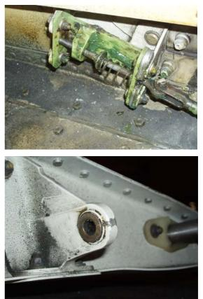
Investigators opened and closed the slide system several times according to the procedure described in the Boeing Aircraft Maintenance Manual (AMM) 25-65-09. The system functioned normally and the carrier and compartment door was found satisfactorily locked at all attempts.
