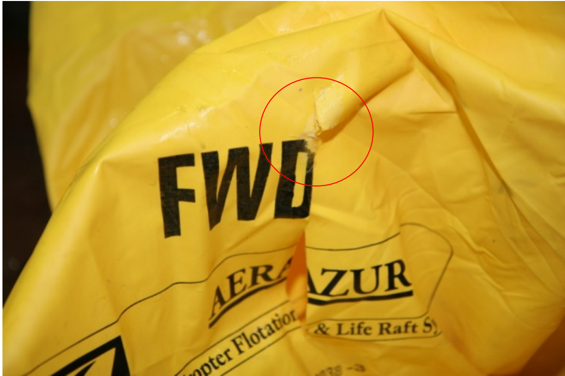
Figure 4: Damaged (deflated) right front float
