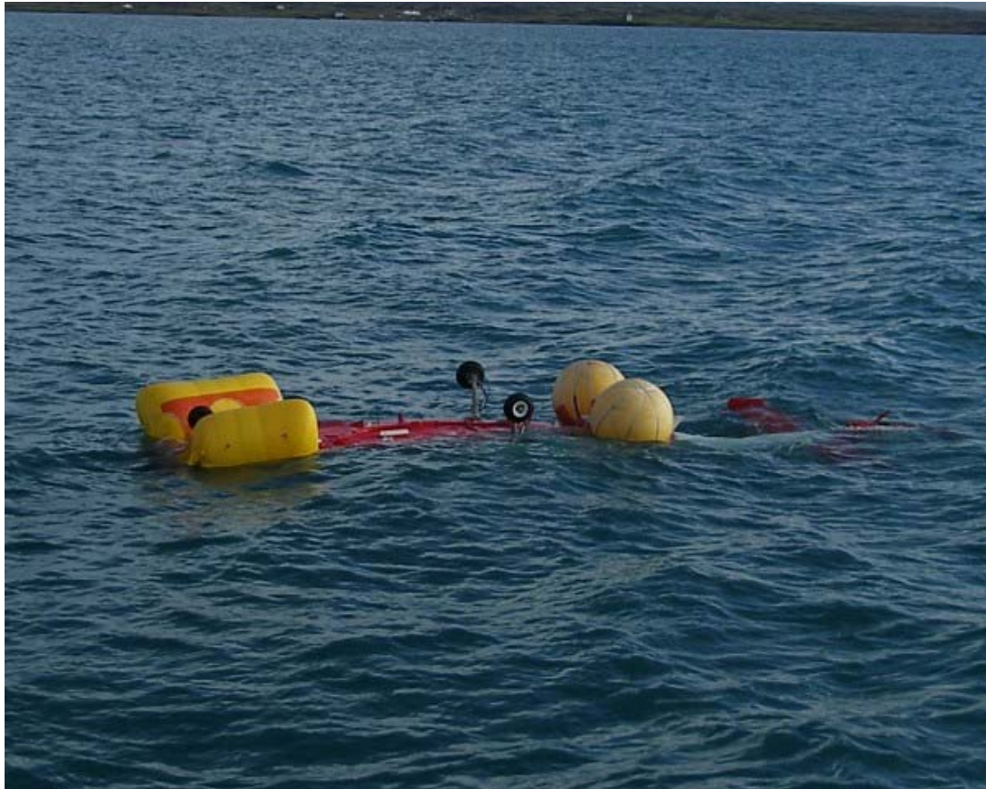
Figure 1: The aircraft capsized approximately 18 minutes after ditching
