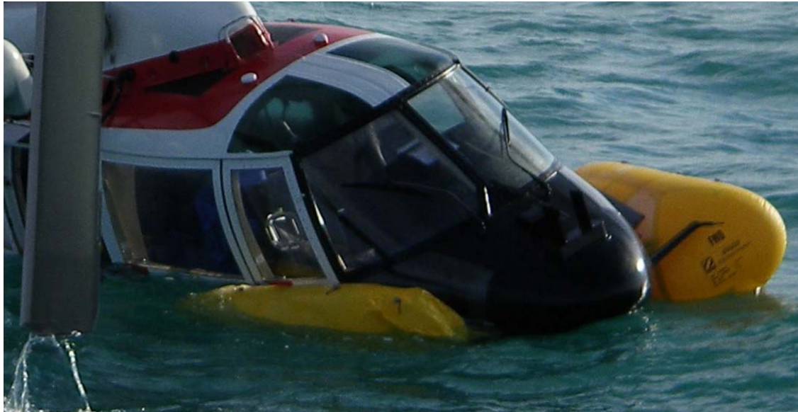
Figure 3: Aircraft with right front float deflated
