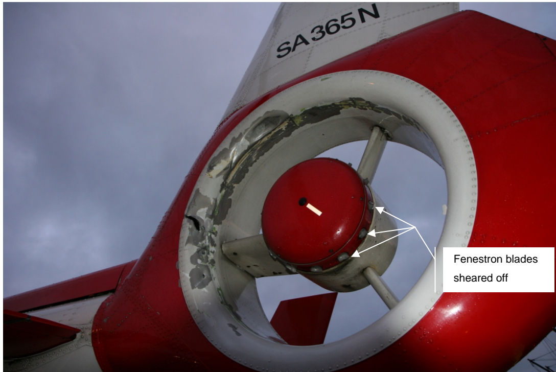
Figure 2: All fenestron (tail rotor) blades sheared off
