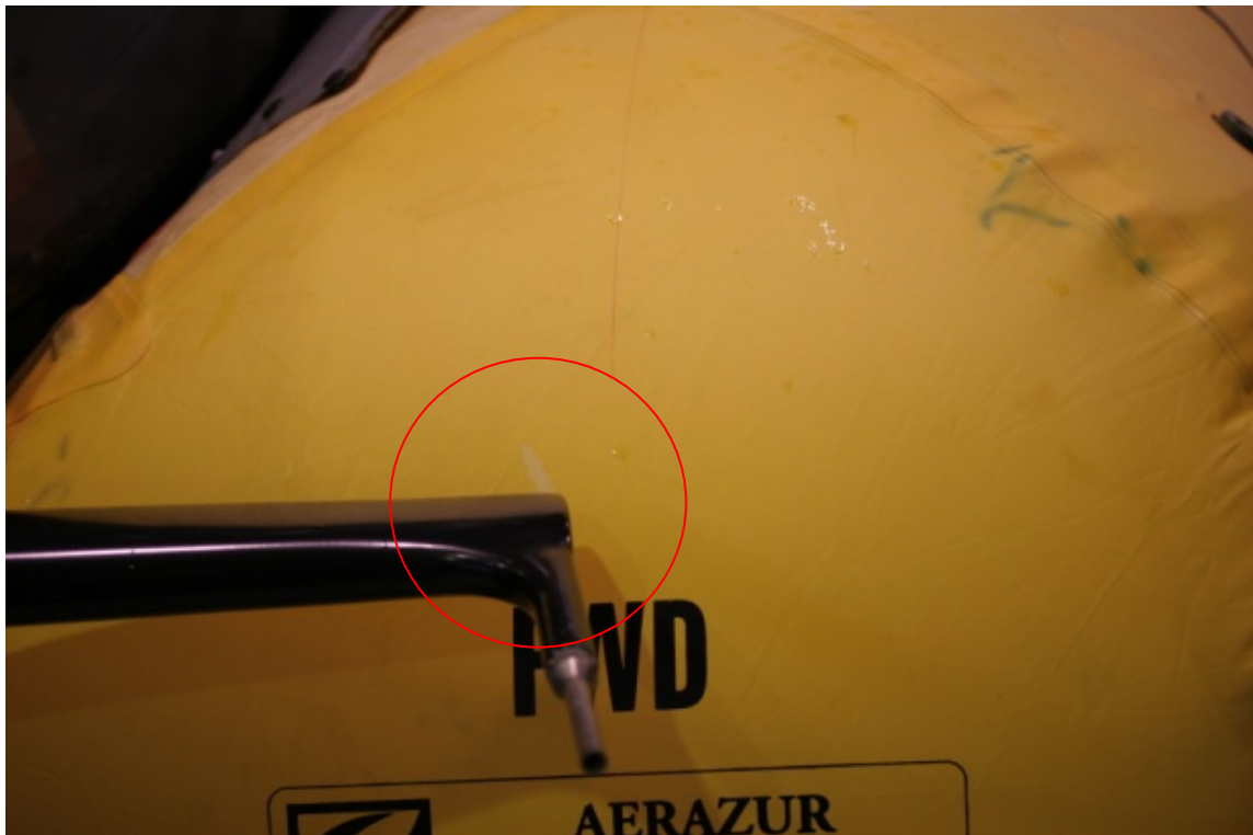
Figure 5: Scratches on left front float (not deflated)
