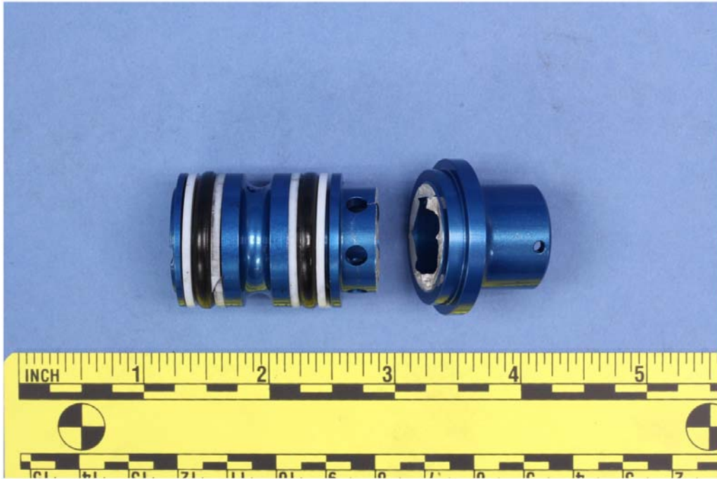
Figure 11: Fractured Blocking and Thermal Relief Valve Housing
